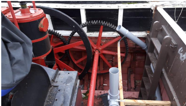
Engine room aft starboard, rotten detached bulwark
